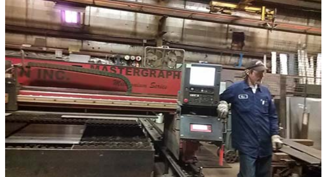
One of the operators fired up the plasma cutter.
