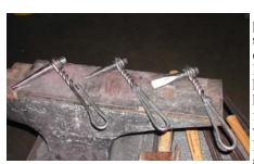
The day will include: preparing a punch, a slitting chisel, and a drift. These are normal length (6 to 8 inches) hand held tools without handles. We will be hand forging as individuals. We will heat treat using oil. Material used will be GM automotive coil spring
