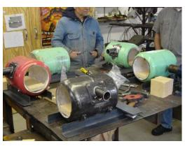
fiber, coated with a cementuous finish for durability. Fire brick will be used for the floor and sliding doors on each end, making it possible to pass the stock through, to heat the center of a work piece. The forge sits in a saddle, and it bolted to it for stability. This forge is a simple, economical forge that is easy to transport and fun to use.
