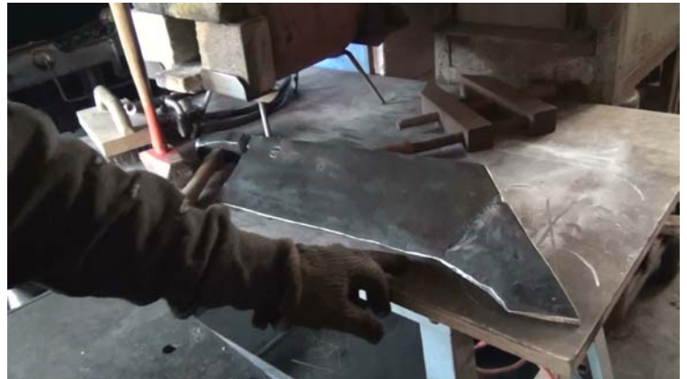
The photo above shows a finished plow share, edge and point restored, ground, and polished.
