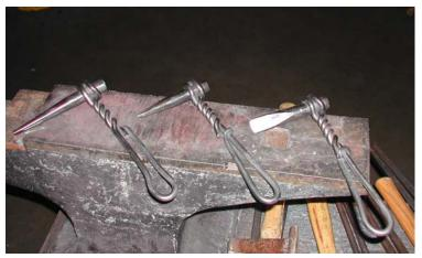
The exercise will include forging and basic heat treatment of the tools. Forge in the morning, heat treat and install handles after lunch.
