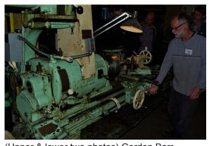
(Upper & lower two photos) Gordon Barr demonstrating on a lathe, where he is cutting a taper.
