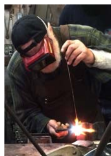
Bill the Welder© demonstrating vertical welding
