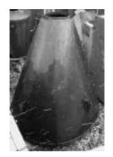
Learn to measure for, lay out, and build an updraft hood for your forge. We will make and use cardboard templates to achieve the layouts of the complicated geometrical shapes, without resorting to trigonometry! One actual hood will be constructed out of 14ga steel using a plasma cutter and MIG welder. This hood will become part of a raffle prize at this year's Madness. Other designs can be discussed. If you bring measurements of your forge, you may be able to complete your own templates.
