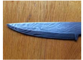
Pattern-welded steel "Damascus"
