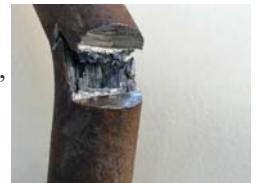
Break Test on 5/8" Rod
