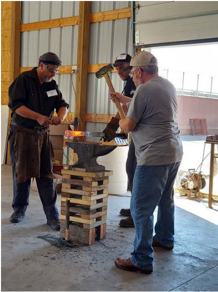
2021 Fall Conference demonstrator Doug Swenson worked with strikers Derrick Phillips and Michael Quackenboss. On this particular photo they are hot cutting the upset end of a 2” round bar of 1045 to be finished as a Viking era stump anvil.
