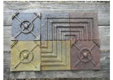
Bronze castings right out of the molds. (After you remove the sprues and vents, this is your take-away).
