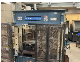
55-ton bending press for testing welds.
