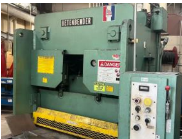
This metal shear can cut a 4 foot piece of 1/2" steel without a problem.
