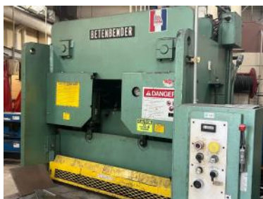
This metal shear can cut a 4 foot piece of 1/2" steel without a problem.
