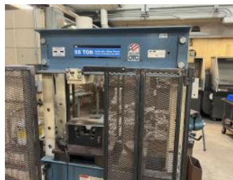
55--ton bending press for testing welds.
