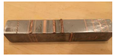
Test piece of 1018 with copper wire inlay
