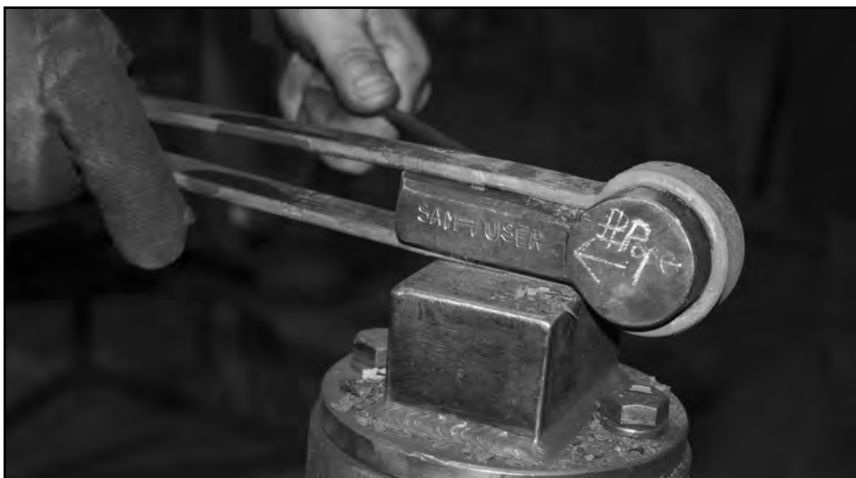
Tool for forming the spring portion of a spring swedge. Sam-Fuser #Pope
