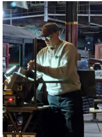
Bob Brown demonstrated his "Homemade Rotary Welding Positioner" for welding round/ circular objects. i.e. pipe, flanges, cylinders etc.
