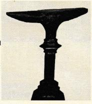
leaf spring and welded along the top of the two horns, after which they will be forged to final shape. The spring steel face should be hard enough without heat treating. The reinforcing cheeks will offer space for touch marks, initials, or decorative ornamentation.
